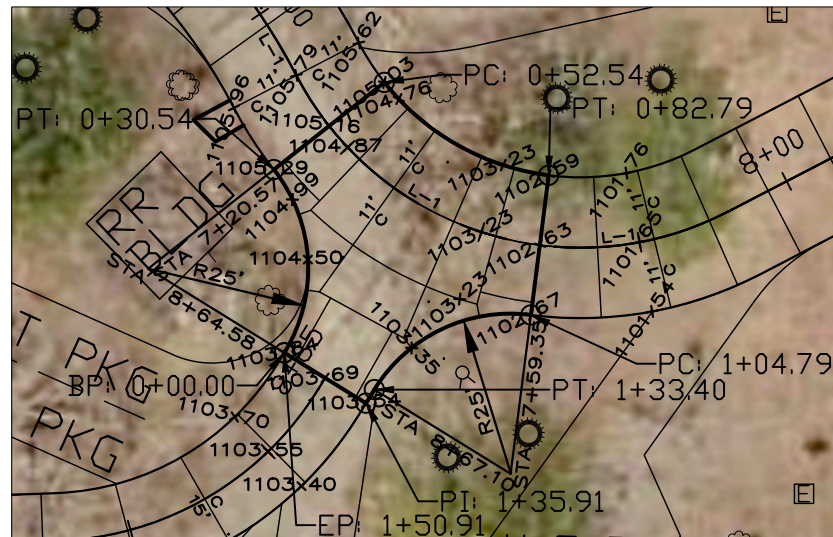
INTERSECTION DETAIL MAIN CAMPGROUND ROAD & WEST ROAD SEE BELOW FOR EDGE OF PAVEMENT CONTROL
